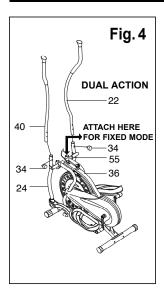
You can easily switch your Right and Left Handlebars (No. 22 & No. 40) between the dual-action mode and the fixed mode during the fixed mode during your workout.
